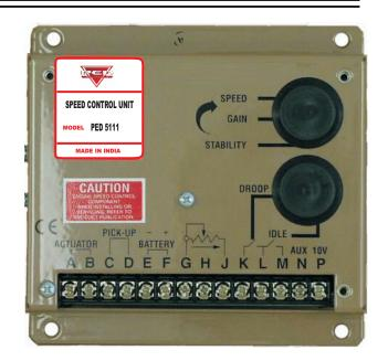
When a speed sensor signal is received by the controller, the signal is amplified and shaped by an internal circuit to provide an analog speed signal. If the speed sensor monitor does not detect a speed sensor signal, the output circuit of the speed control unit will turn off all current to the actuator.
